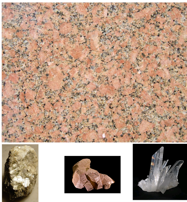
Figure 1: Granite (top) and its components: mica (left), feldspar (center), and quartz (right)
