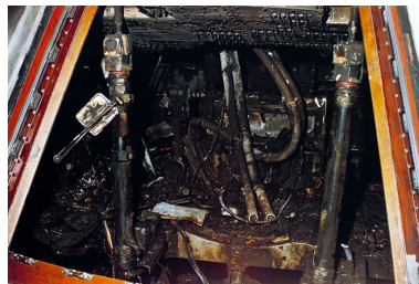
Figure 6: Appollo 1 cabin's interior after fire.
