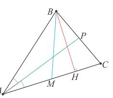
An **angle bisector** of a triangle is a straight line through a vertex which cuts the corresponding angle in half.
