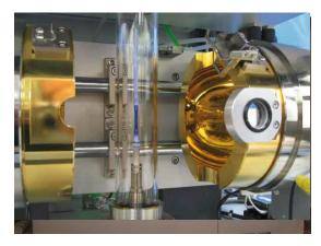
will hold for all rays out of the source. Alternatively, a cylindrical mirror with elliptical cross-section can be used to focus light from a linear fluorescent lamp along a line of the paper; such mirrors are used in some document scanners. 3D elliptical mirrors are used in the floating zone furnaces to obtain locally high temperature needed for melting of the material for the crystal growth.
