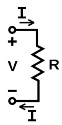
• R is Resistance of the wire. Measured in Ohms  $[\Omega]$ .  $1\Omega=1V/A$
