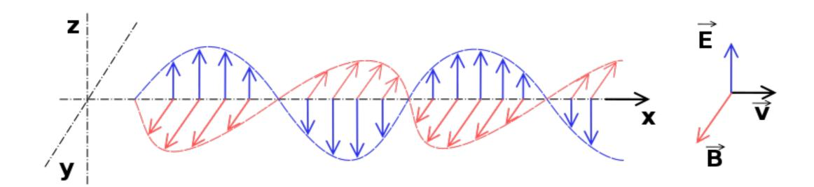
E(t) -> B(t) -> E(t) -> B(t) -> .... - oscillations of E and B propagating in space. **Electromagnetic Wave**.
