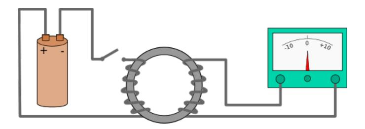
Electric field (from battery) -> Electric force -> Charges move (current) -> Changing magnetic field in the ring -> Electric field in the second coil -> current in the second coil
