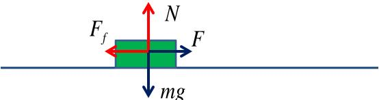
• STATIC FRICTION Imagine that you try to move a block on a floor by pushing it with force F. The block does not move because of static friction with the floor. That force oppose motion, and will be equal to F to make sure that the block is at rest. However it cannot be bigger than certain maximum value:
