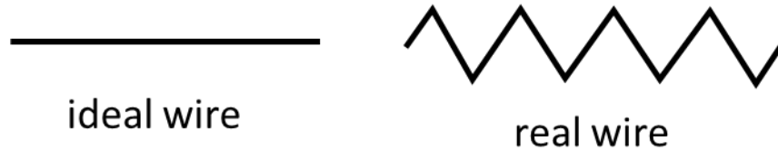
Figure 1. Ideal and real wires.
