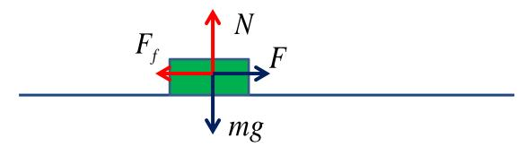
STATIC FRICTION Imagine that you try to move a block on a floor by pushing it
