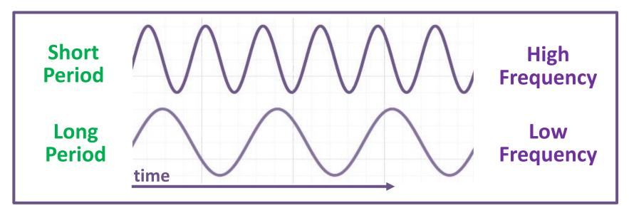
PERIOD (T): The time it takes to make one complete vibrational cycle. FREQUENCY (f): number of waves per second.
